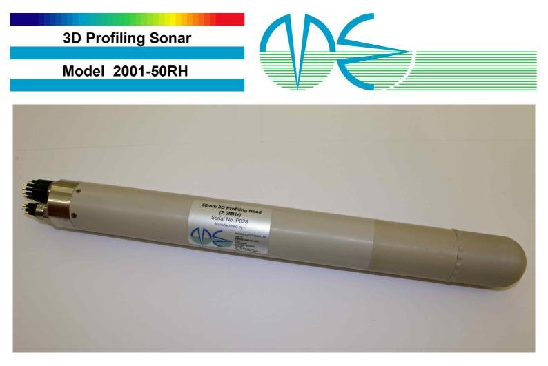
The 3D Profiling Sonar Model 2001-50RH is designed to operate long term in radioactive ponds and settlement tanks and gather high resolution bathymetry data. Manufactured in PEEK and only 50mm in diameter the unit can be installed through the smallest of access points. Multiple units can be linked together and controlled via Ethernet to enable large areas to be fully mapped. The windows software allows images to be merged to produce a single point cloud picture.
